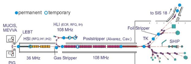
Figure 1: Overview of the UNILAC and the emittance measurement device positions.
