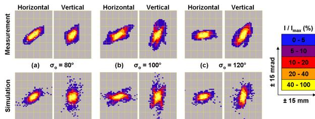
Figure 8: Experimental (top) and simulated (bottom) transverse emittances behind Alvarez I tank for a 7.1 MeV  $^{40}\text{Ar}^{10+}$  beam. At  $100^\circ$  phase advance the fourfold symmetry in the phase space distribution is clearly visible.
