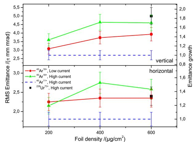
Figure 6: Effect of ion stripping by a carbon foil on the transverse emittance, measured for three different foil densities. The dashed line indicates the unstripped beam. Exemplary data points for  $^{238}\text{U}$  are added.
