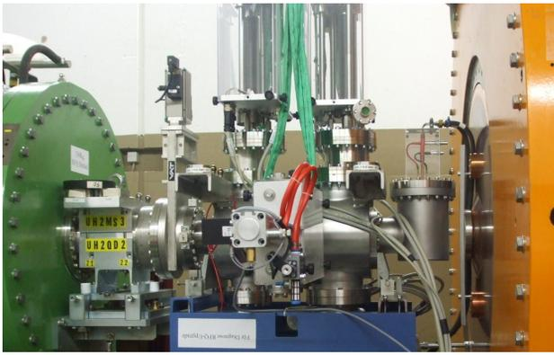
Figure 3: A buncher cavity had been removed to install the emittance device between the HSI RFQ (green, left) and IH1 (orange, right).
