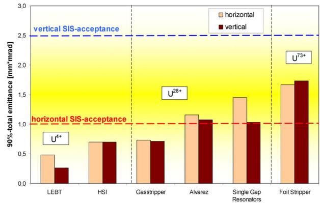
Figure 5: Emittance growth along the UNILAC for a  $^{238}\text{U}$  beam. Indicated are the horizontal and vertical acceptance limits of the SIS 18 with respect to FAIR operation.
