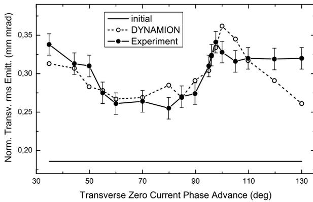
Figure 7: High current transverse emittance growth along the Alvarez DTL as a function of the (zero current) transverse phase advance: Simulated  $\circ$  and experimental  $\bullet$  data. The straight line indicates the reference emittance at the DTL entrance.
