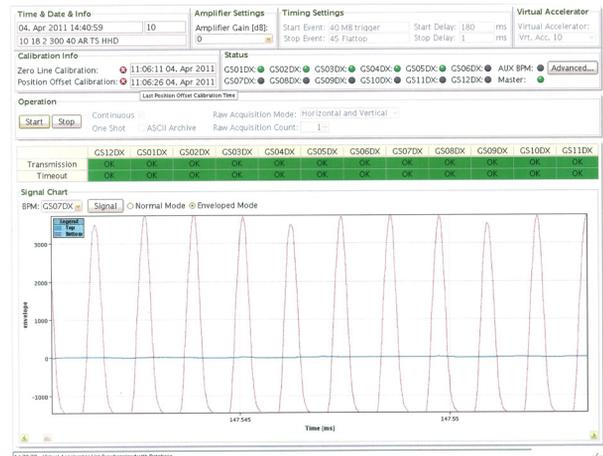
Figure 1: TOPOS in raw data mode, showing longitudinal bunch profiles of four bunches in the GSI synchrotron over several turns.
