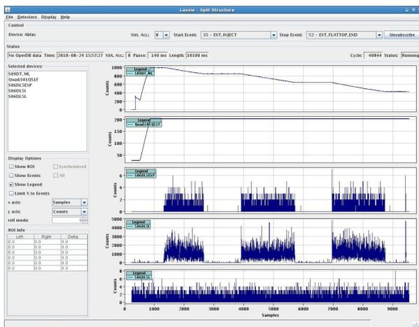
Figure 2: LASSIE screenshot of a sequential slow extraction of the GSI synchrotron, showing the following machine parameters (top to bottom): beam current in the ring, magnet ramp and signals of three beam loss monitors.
