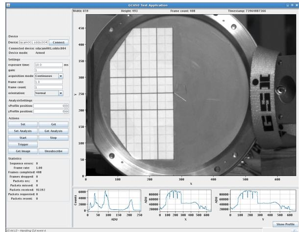
Figure 3: GigE camera readout with FESA. The screenshots shows the prototype GUI with an image of a scintillator screen test installation.
