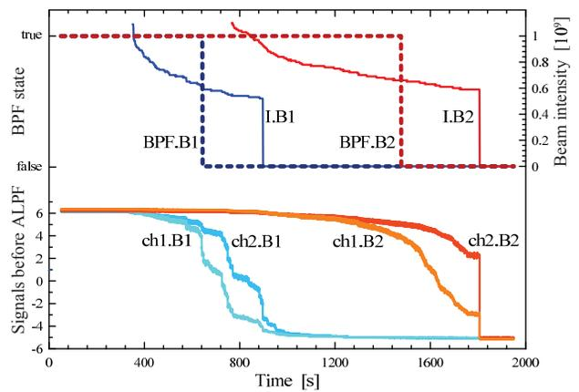
Figure 6: Beam measurement of the BPF system thresholds.
