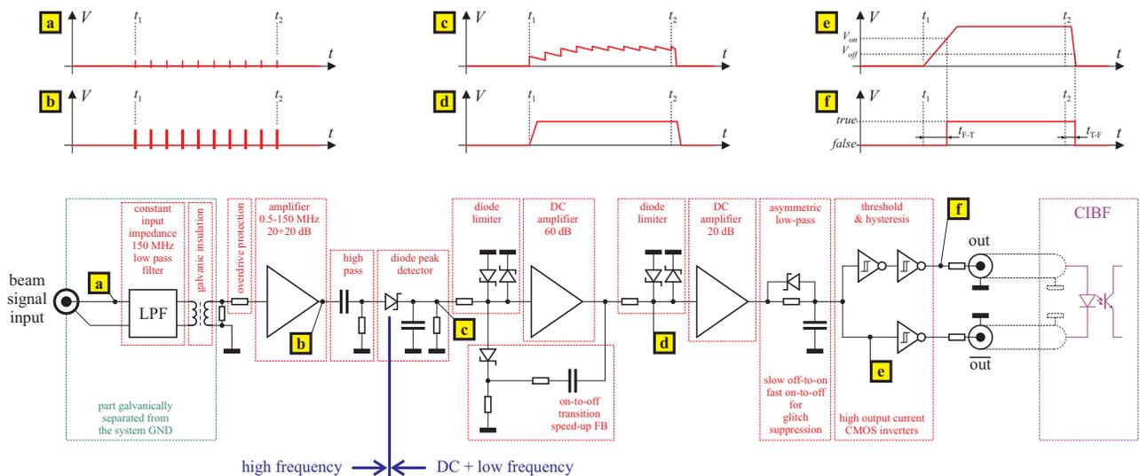
Figure 2: Functional diagram of one channel of the beam presence flag front-end with sketches of signal waveforms in the most important nodes of the circuit. Each FE unit has 4 identical channels.
