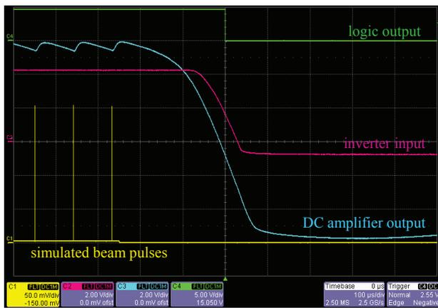
Figure 3: Signals for the worst case ‘true’ to ‘false’ transition. The actual FE input voltage is 40 dB smaller.
