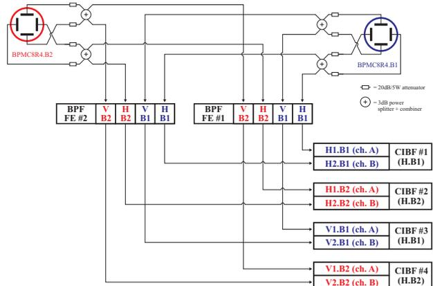
Figure 1: Architecture of the LHC beam presence flag system based on BPM signals.
