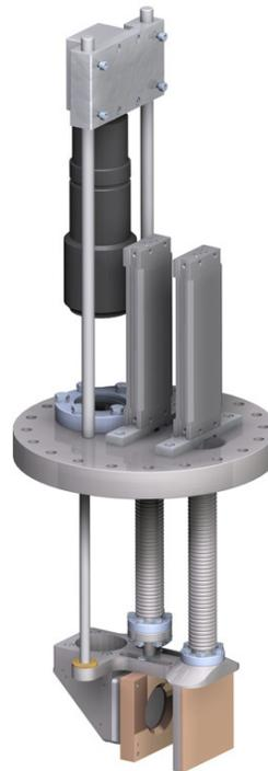
Figure 5: Pepper-pot emittance meter with water-cooled shutter based on CF160 flange.
