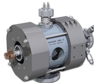
Figure 1: Dresden EBIS-A, based on permanent magnets.
