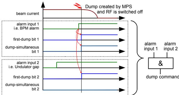
Figure 4: Dump-Simultaneous-Alarm bit: is only set, if the dump was generated simultaneously with changing to active state of this alarm input. First-Dumping-Alarm bit is set for each combined input which had led to the dump.
