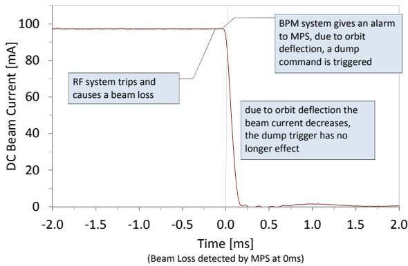
Figure 5: RF failure before the beam loss (rule 1).
