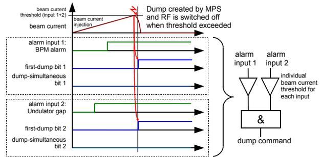
Figure 7: Dump by exceeding the beam current threshold of a BPM alarm input when orbit alarm already active and undulator gap is closed while increasing beam current during injection (rule 6).
