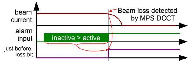
Figure 2: Just-Before-Loss-Alarm bit.
