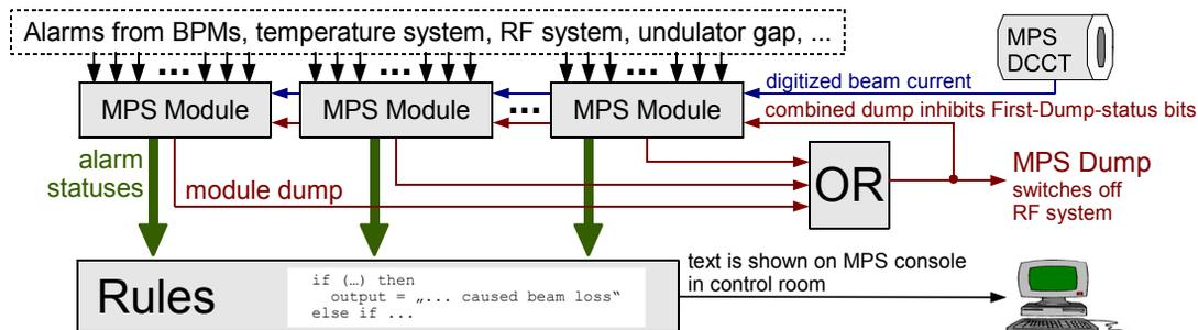
Figure 1: Signal flow inside the MPS.
