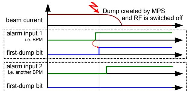
Figure 3: As the First-Dump-Alarm bit is system wide, it is only set for alarm input 1. Alarm input 2 became active after the first-dump-alarm bit had been set for alarm input 1 (see combined dump in Fig. 1).
