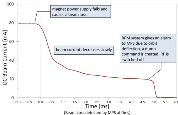
Figure 6: Magnet power failure causes the beam loss (rule 2), BPM alarm and dump afterwards.
