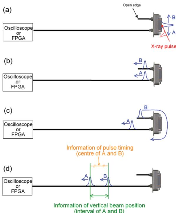
Figure 7: Sketches of the behaviour of the pulse transmission with the open end.
