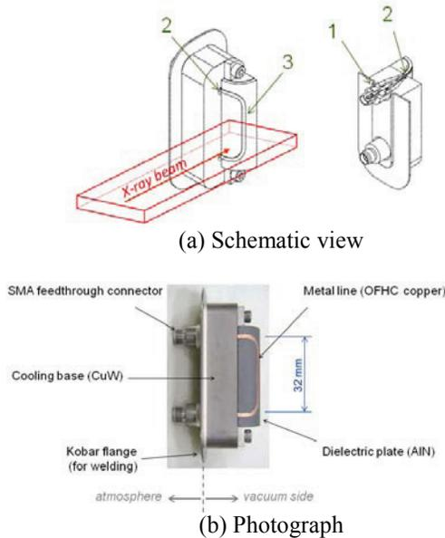
Figure 3: Structure of the detector head.
