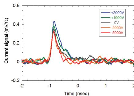
Figure 6: Pulse shapes with various high voltages.
