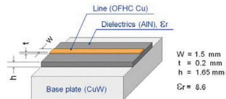
Figure 2: The basic structure of the detector head with a microstripline structure.
