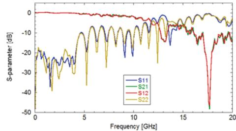
Figure 4: S-parameters of the detector head.
