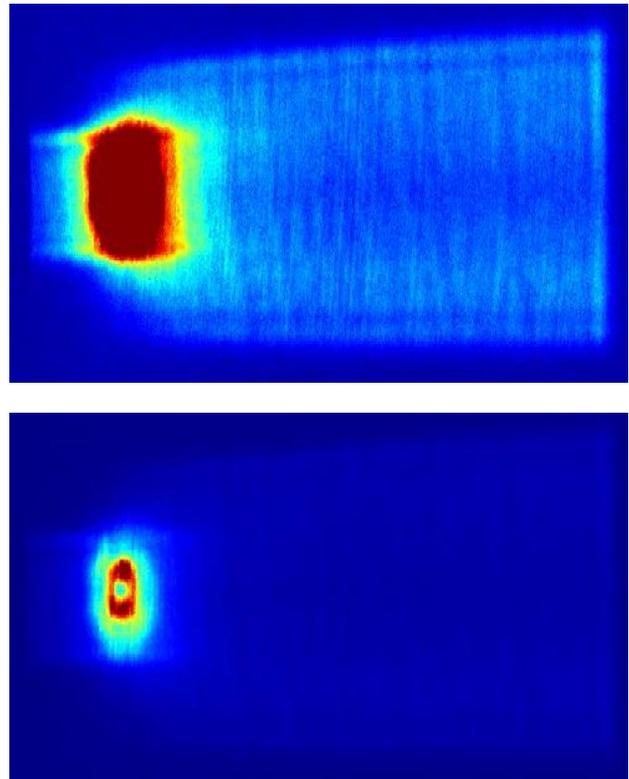
Figure 5: Image of the projected visible light (no colour filters) onto a screen at 8m from the dipole source.
