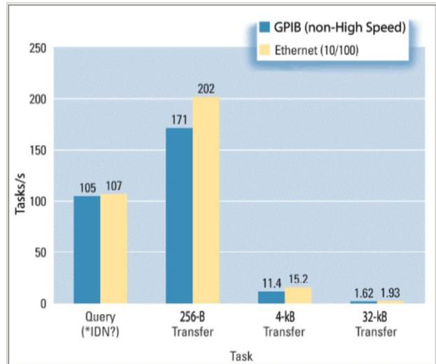
Figure 3: Ethernet 2% to 34 % faster than GPIB for queries and transfers [3].
