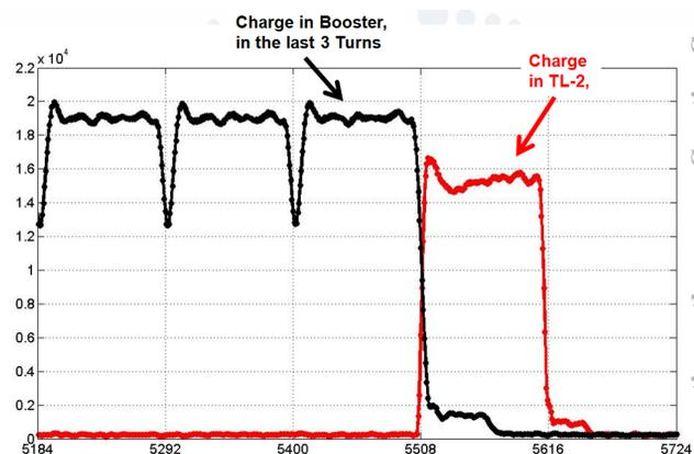
Figure 1: Charge outputs of two devices, showing 3 turns of 1µs long pulse in the Booster (black) and the subsequent extracted beam in the TL2 (red).
