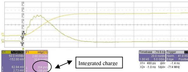
Figure 2: LINAC Short Pulse - Green: ICT output pulse Yellow: Surface integral of ICT output pulse.
