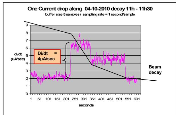
Figure 4: Diagnostics from Ethernet-Based DMM Keithley using post triggering data buffer.
