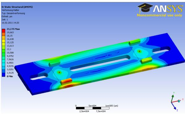
Figure 6: Deformation of the original holder plate.
