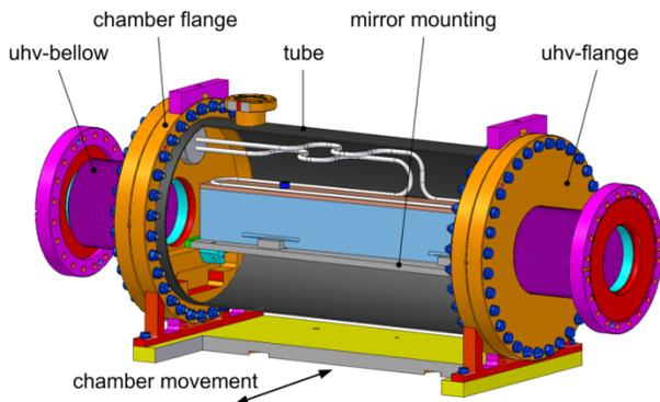
Figure 1: Fast Switching Mirror Unit.
