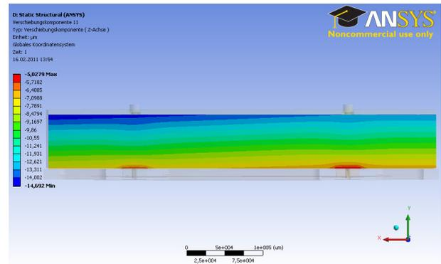
Figure 7: Deformation of the mirror (original).
