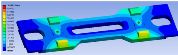
Figure 11: Deformation of the modified holder plate.
