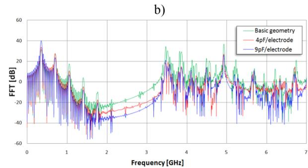
Figure 5: Simulation of between three BPM models: a) output voltages, b) spectra versus capacitance.
