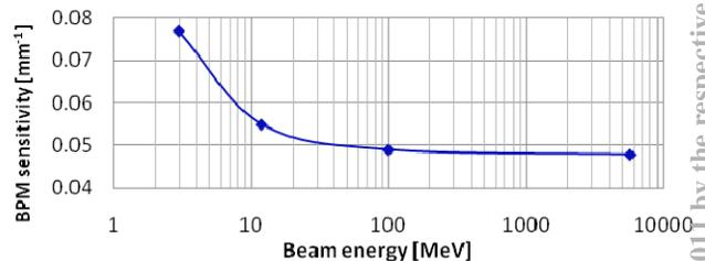
Figure 6: Estimated sensitivity at 352MHz as a function of beam energy.
