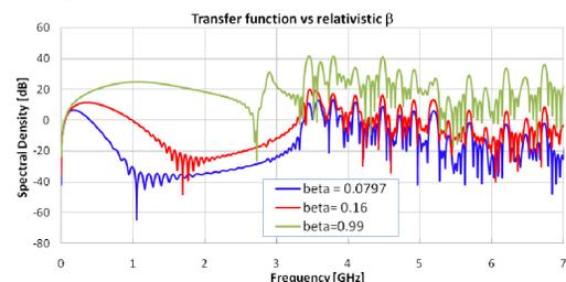
Figure 2: BPM transfer function for different beam velocities.
