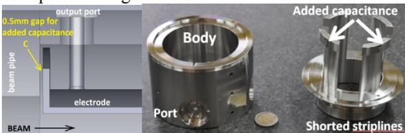
Figure 4: Left: Principle of added capacitance. Right: Body and electrodes with added capacitance before electron welding.
