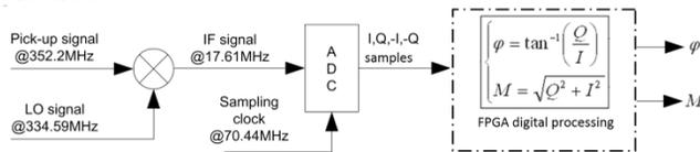
Figure 7: I/Q acquisition principle.
