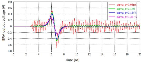
Figure 3: BPM output signals from a run with a 12 MeV-single bunch. The  $1\sigma$  bunch length span is 0.05-0.35 ns.
