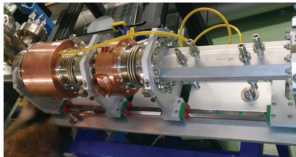
Figure 1: Beam diagnostics components in Sector 2. From left to right, the DCCT, AE, FCT, and a stripline BPM.
