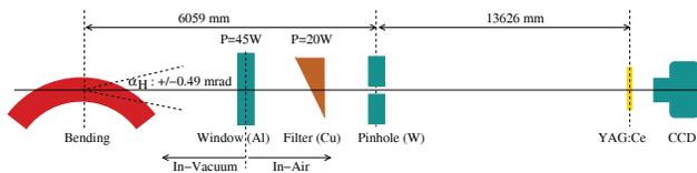
Figure 8: Schematic lay-out of the pinhole camera.
