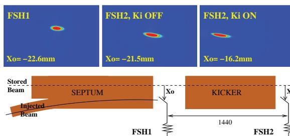
Figure 2: Sketch of the FSHs location at injection straight (bottom), and beam image at FSH1 (left), at FSH2 with kicker OFF (middle) and ON (right).
