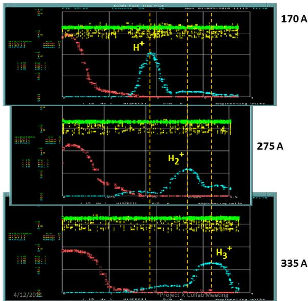
Figure 2: Measurement of ion source species content. Plots show Faraday cup intensities versus spectrometer magnet current. The LEBT downstream solenoid has been optimized to focus individual species to the east Faraday cup. Red curves show west Faraday cup current (straight line) while blue curves show east Faraday cup current (spectrometer line).
