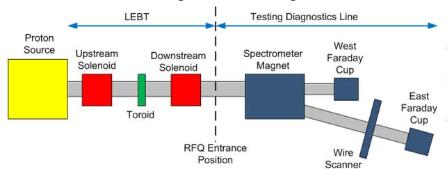
Figure 1: Ion source and LEBT measurement setup.
