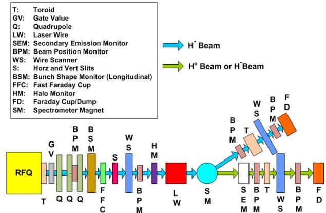
Figure 4: Block diagram of HINS improved diagnostics line for RFQ measurements and future HINS accelerator configurations.
