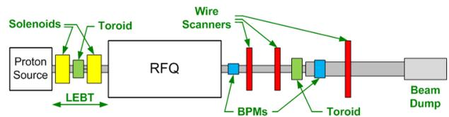
Figure 3: HINS beamline and diagnostics for initial RFQ measurements.
