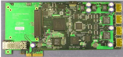
Figure 4: The PCIe FMC carrier developed at CERN.
