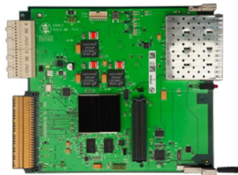
Figure 10: A MTCA .4 FMC carrier developed at DESY
