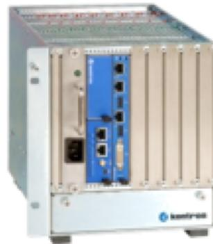
Figure 9: A uTCA crate. In the 1st slot there is the power supply, in the second the MCH and in the 3rd a crate PC.
