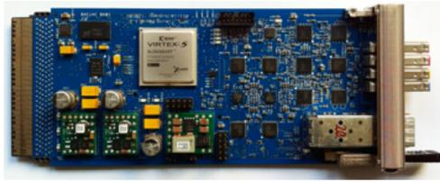
Figure 7: A uTCA board for a timing distribution system developed in a collaboration between the University of Stockholm and DESY.
