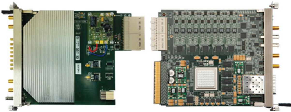
Figure 1: Analog-to-digital converter board SIS8300 with RTM.
