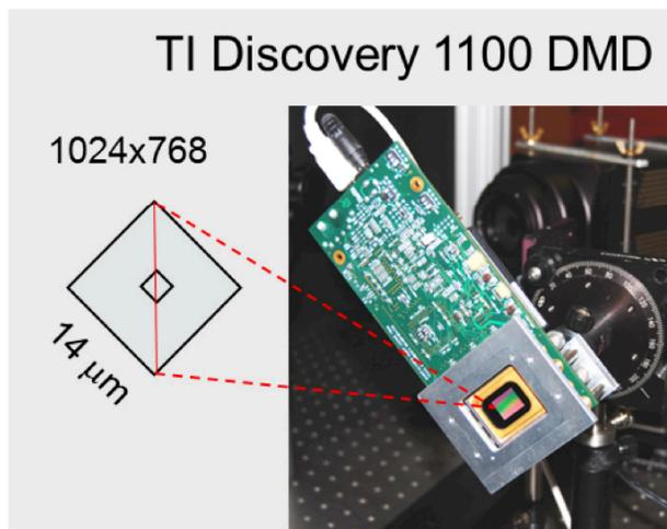
Figure 13: The Texas Instruments digital micro-mirror array transmits the transverse beam distribution without the beam core, i.e., the beam halo.
