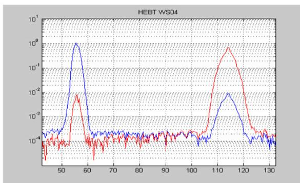
Figure 7: During a single wire scan, there was coupling between the wire scanner horizontal (red trace) and vertical (blue trace) wires. This coupling is being eliminated, thereby increasing the wire scans dynamic range.
