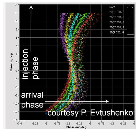
Figure 10: The ERL acceleration cavities are first set to accelerate beam in such a way so as to minimize beam space charge effects.
