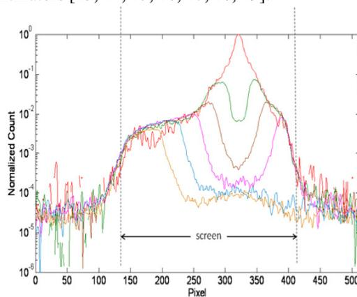
Figure 14: This graphic shows a transverse projected distribution of the beam core and halo (distribution edges) using a digital micro-mirror array.
