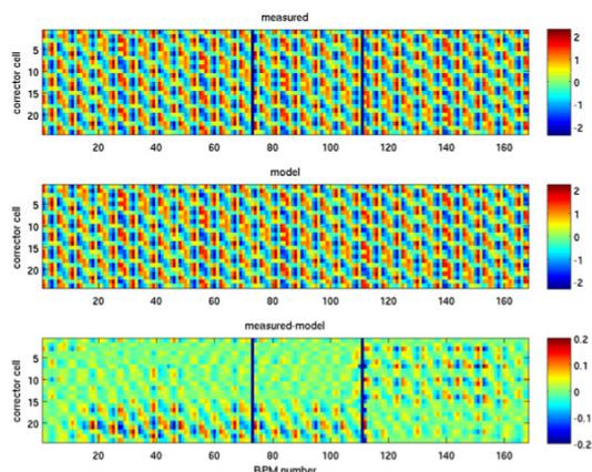
Figure 12: Using this injected moving beam bunch techniques, typical Diamond Light Source measured (top), modelled (middle), and resultant corrector response matrices (bottom) are graphically displayed.
