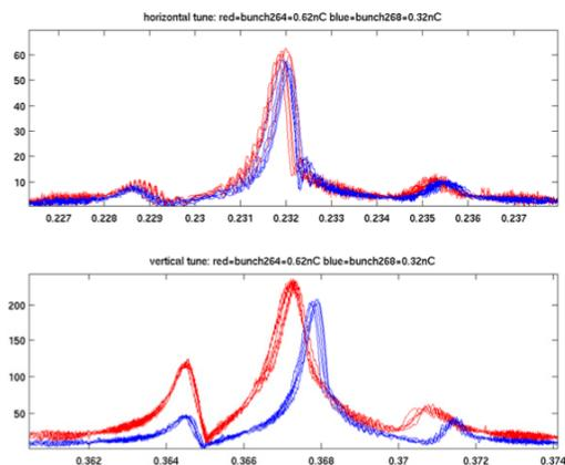
Figure 11: Horizontal (red) and vertical (blue) tune measurements of the sinusoidally disturbed beam for the Diamond Light Source ring.
