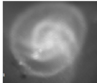
Figure 9: This graphic of a viewscreen shows the two-dimensional shape of multi-species extracted beams 1 m downstream.
