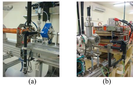
Figure 4: (a) Linac screen monitor and (b) test transport line screen monitor.
