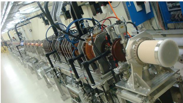
Figure 1: TPS 150 MeV linac being installed and commissioning at accelerator test site.
