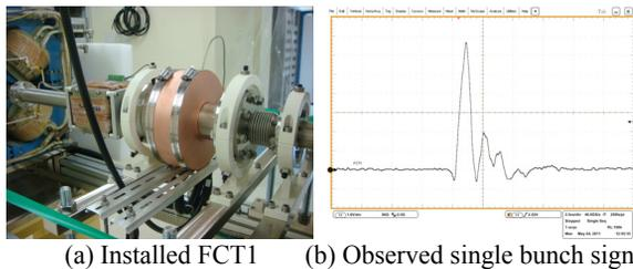
Figure 7: FCT and its signal at the test transport line.
