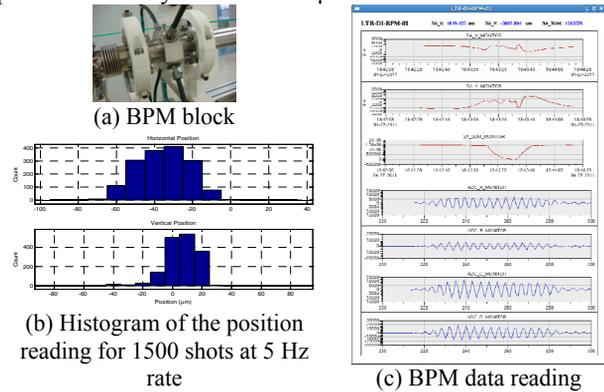
Figure 8: BPM block and data at the test transport line.
