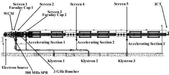
Figure 2: Diagnostic devices layout for the TPS linac.
