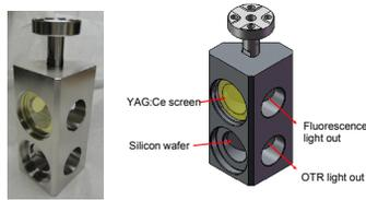
Figure 5: Dual-position screen assembly. The upper part is YAG:Ce working in normal incident, fluorescence is reflected to camera horizontally by a mirror installed the 45° position. The silicon wafer coated with aluminium layer install at 45° position used as OTR radiator is in the lower part.
