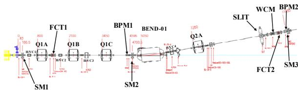
Figure 3: Functional block diagram of the temporary transport line for acceptance test.
