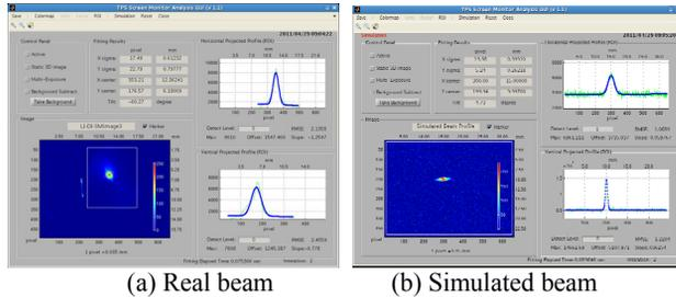
Figure 6: Screen monitor analysis user interface.
