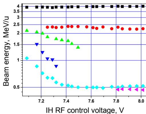
Figure 4: Energy spectra of the ions coming out of IH depending on RF amplitude for a fixed phase of  $235^\circ$ . Black squares shows primary beam, cyan diamonds trends continuously down to the design energy of 0.5 MeV/u. Blue circles, green up-side triangles and blue down-side triangles stand for particles with variable intermediate energy.
