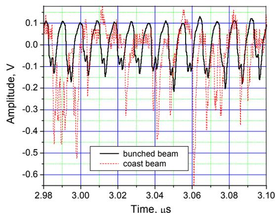
Figure 1: Signal from the polycrystalline diamond detector. The solid line shows the bunched beam, the dashed line the beam without bunching.
