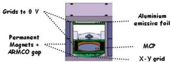
Figure 7: Head design details of the secondary emission foil profiler.
