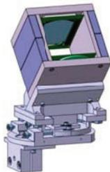
Figure 6: Head of secondary emission foil profiler.
