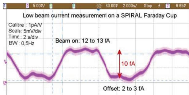
Figure 5: Low beam current measurement.
