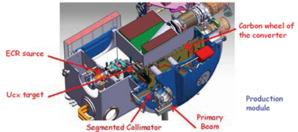
Figure 3: Horizontal cut of the production module.
