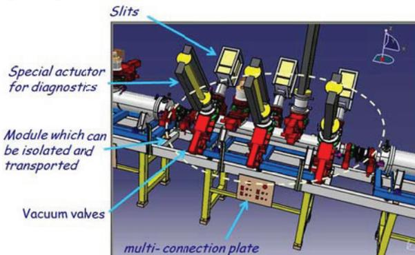
Figure 2: Example of a module in the yellow zone.
