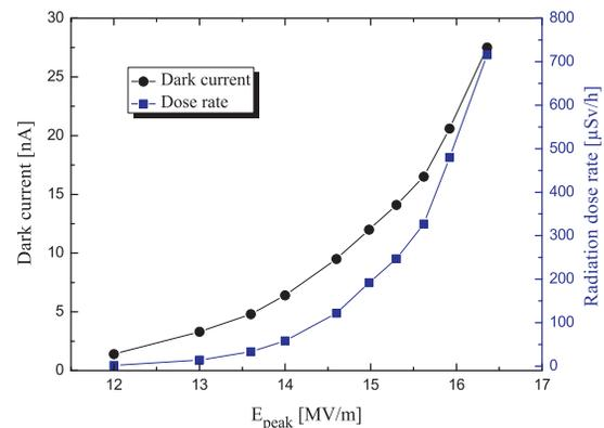
Figure 3: Dark current measured with the Faraday Cup and proportional counting tube versus electric field gradient.
