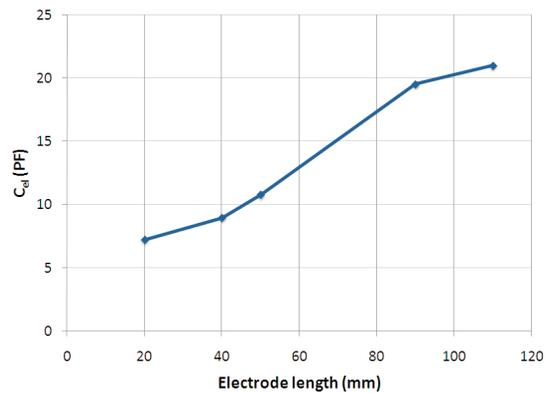
Figure 6: Capacitance of one electrode as function of the length.
