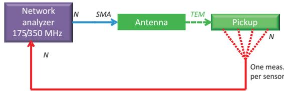
Figure 2: Scheme of the BPM wire tests using a network analyzer.
