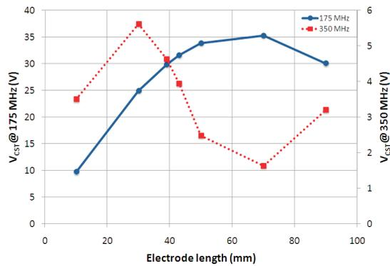
Figure 4: Response of one electrode as function of the length.
