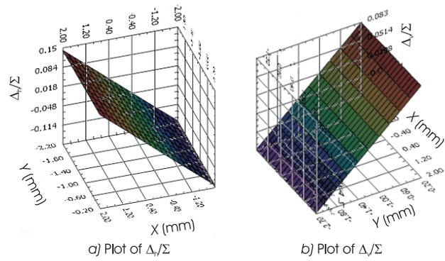
Figure 3: 3D plots of the response of the CBPM at 350 MHz: a) Horizontal delta over sum, b) Vertical delta over sum.
