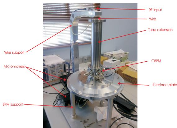
Figure 1: The CIEMAT BPM test bench.
