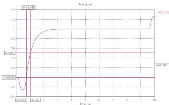
Figure 5: Time domain reflection response of one sensor to a step stimulus.
