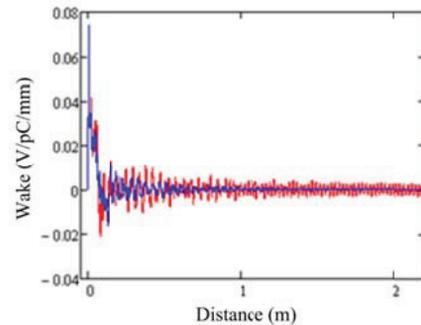
Figure 7: Wake, damped (blue) and undamped (red).
