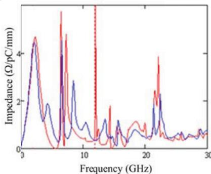
Figure 6: Transverse impedance for undamped (red) and damped (blue) stripline.
