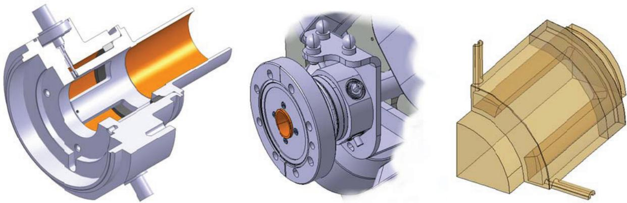
Figure 2: Drive Beam BPM, BPM inserted into drive beam quadrupole, and GdfidL model.
