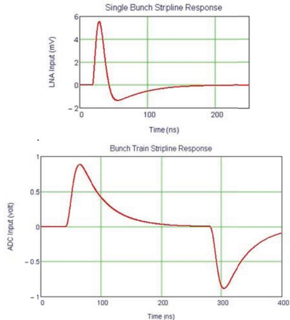
Figure 4: Simulated single bunch and train response after processing filters.
