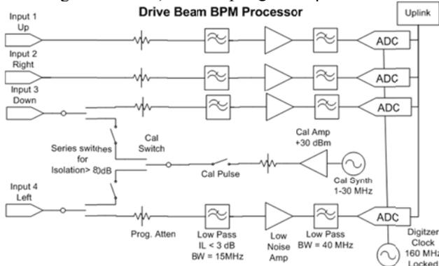
Figure 3: Drive Beam BPM Processor.
