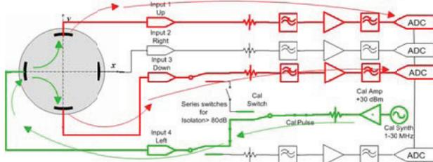
Figure 5: Y axis calibration signal flow.
