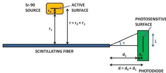
Figure 2: Geometrical proportions of the light cone emitted by the fiber.
