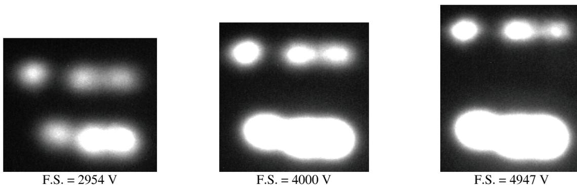
Figure 3: CCD images (upper spots) of the light produced in the F.S. by 3.5 keV  $H_2^+$  beam for different  $V_{F.S.}$  at fixed MCP (1326 V) and Al plate (-6.4 kV) voltage. Two beam spots of diameter 1 mm each and separated by 2 mm can be clearly seen, suggesting a spatial resolution of 2 mm of the system. The diffused lower spots are due to the Bremsstrahlung photons that are created when the beam passes through the narrow channel of the RFQ. The upper spots shift with the F.S. voltages.
