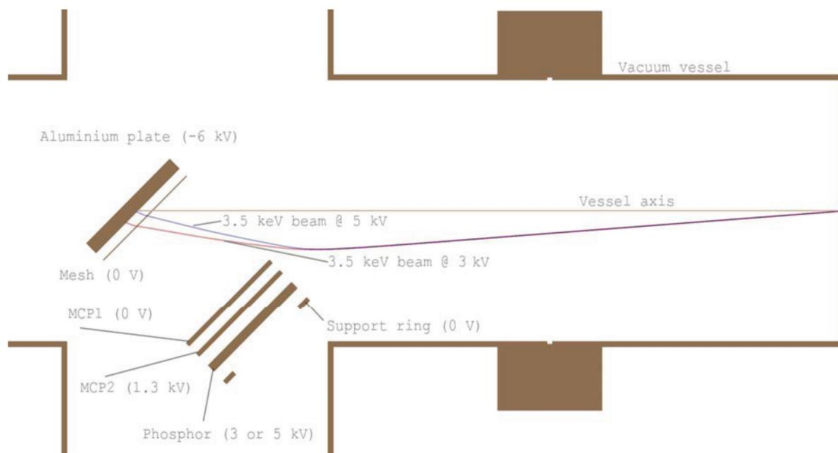
Figure 4. SIMION Calculations for the 3.5 keV  $H_2^+$  beams for different F.S. voltages.
