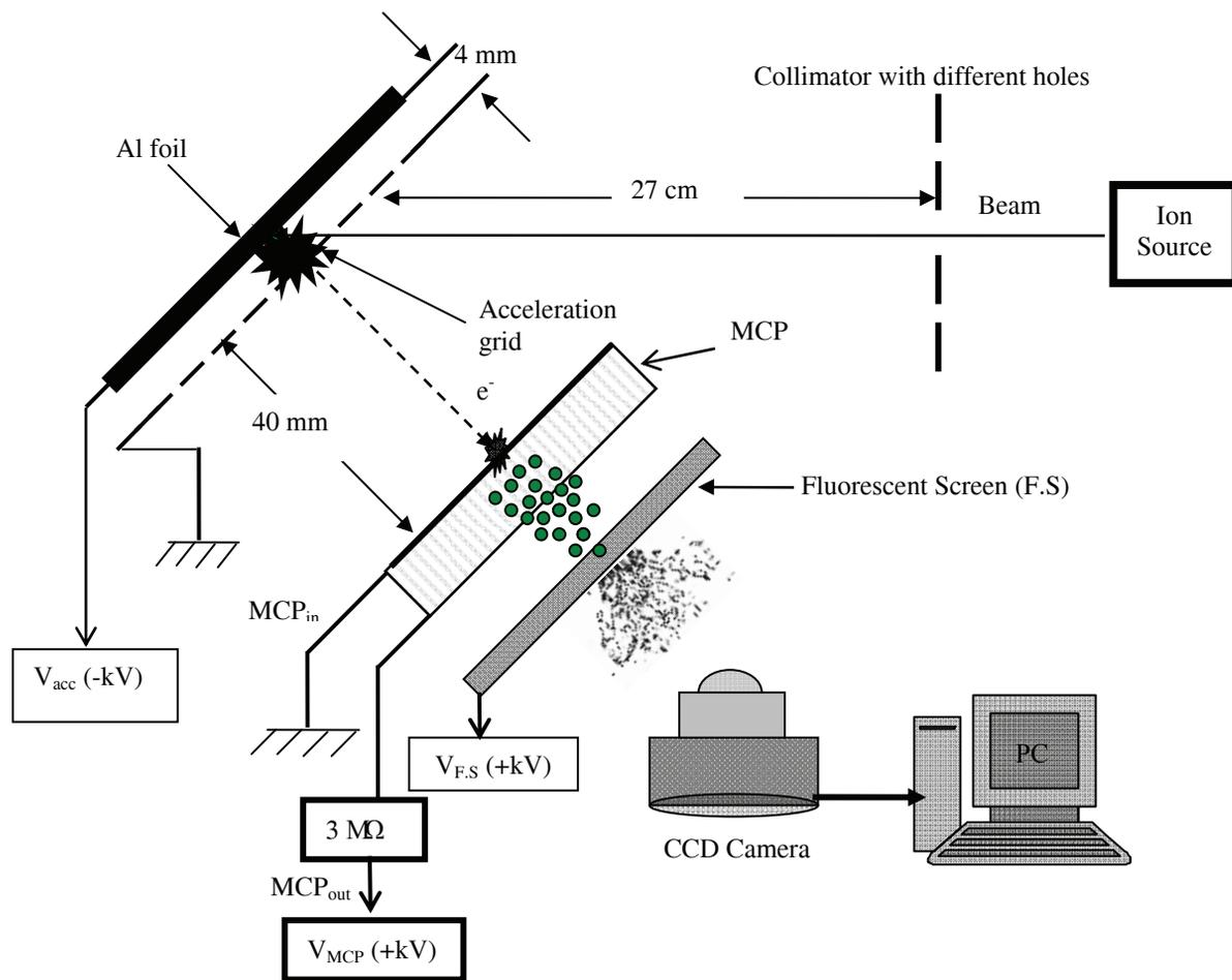
Figure 2: Schematic diagram of the experimental set-up.
