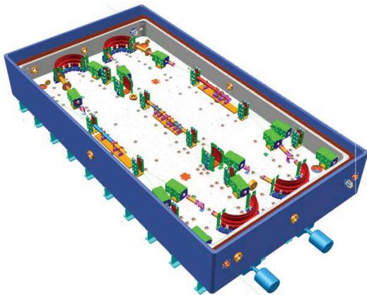
Figure 1: Schematic layout of DESIREE. It consists of two rings of same circumference, 9.2 m, and a common straight section of length 1 m for the merged-beams experiments with ions of opposite charges.
