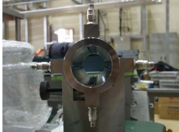
Figure 6: The prototype of BPM.
