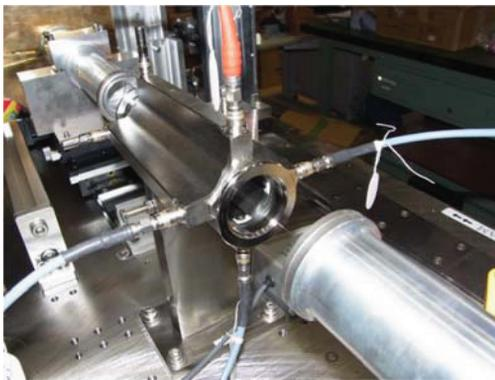
Figure 8: The aspect of BPM calibration with a wire.
