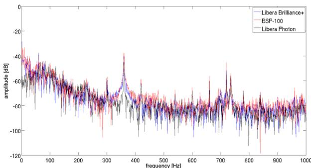
Figure 5: Noise spectrum of three beam position monitors.
