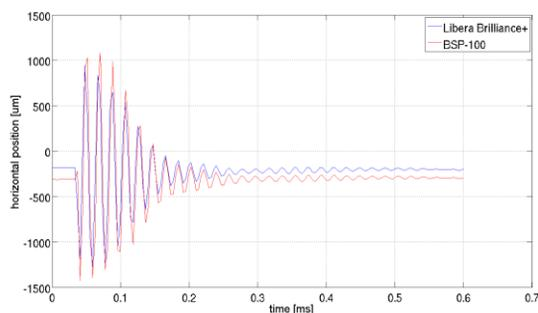
Figure 8: Detailed look at the injection transient during the top-up injection.
