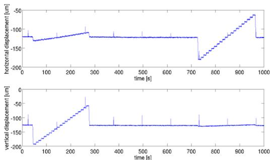
Figure 3: Vertical and horizontal angle bumps.
