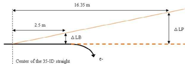
Figure 2: Calculating the displacement of the beam at S35ID:P1 location.
