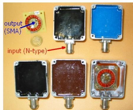
Figure 4: Matching transformers non-encapsulated and encapsulated in epoxy (from left top to down bottom). The order is the same as in Table 1.
