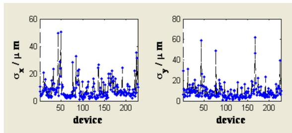
Figure 4: Standard deviation of TbT readings after beam dump during DSC learn phase (same beam properties; note the different scales for both figures).
