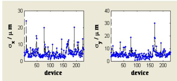
Figure 3: Standard deviation of DSC-optimized TbT readings before beam dump (40 bunches, 55mA, FOFB on, no Top Up).
