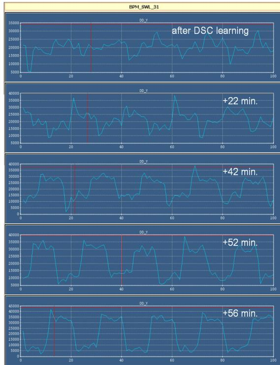
Figure 2: Drift of DSC switching amplitude vs. time (zero beam offset, vertical TbT, 40-bunch time-resolved mode, 80mA (const.), FOFB on, TopUp mode, const. ambient temperature +/- 1° at the electronics).
