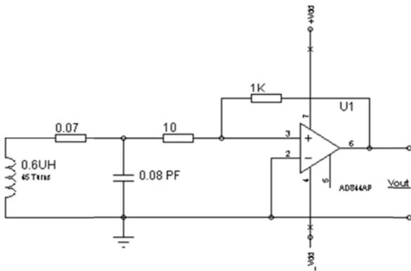
Figure 1: The equal circuit of system.
