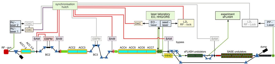
Figure 2: Schematic of the laser-based synchronisation system at the upgraded FLASH accelerator facility.
