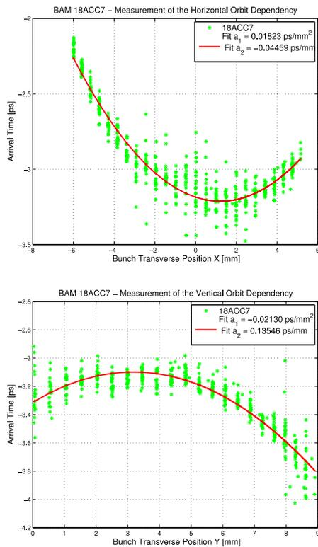
Figure 5: Arrival time vs. beam position in the horizontal (upper plot) and in the vertical plane (lower plot) for BAM No.4, located downstream of the last accelerator module, ACC7
