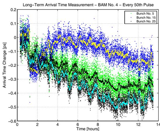
Figure 6: Long-term arrival time measurement with BAM 4. Shown is data from bunches No. 5, 15 and 25 of bunch trains with 25 bunches. Only the last one was used to generate FEL pulses. Those short-term timing oscillations are due to not optimal BBF settings in the first accelerator module ACC1 and are then transported throughout the whole machine.
