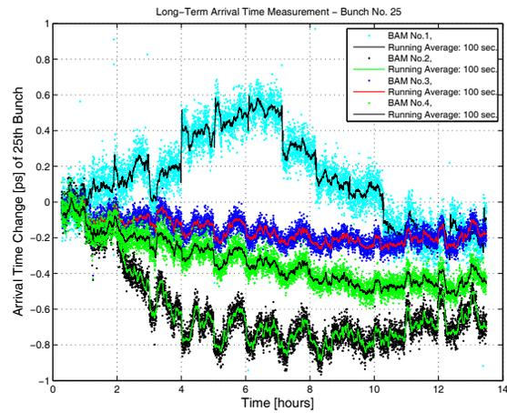
Figure 7: Long-term measurement with all BAMs. Arrival time is stabilised at BAM 2 and 3, while BAM 4 is used as an out-of loop monitor. The arrival time feedback loop on the injector is not yet commissioned.
