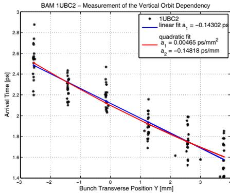
Figure 3: Arrival time vs. beam position in the vertical plane for BAM No.1, located in front of BC2. The arrival time does not depend on the horizontal position for this BAM.
