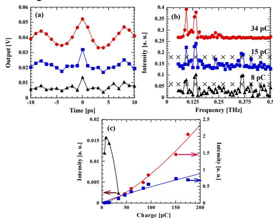
Figure 3: Interferograms near the centerburst position for 34, 15 and 8 pC bunch charges with offsets and factors adjusted for comparison. (b) Frequency spectra for 34, 15 and 8 pC bunch charges with offsets and factors adjusted for comparison. The theoretical frequencies of  $TM_{0n}$  modes (cross) were shown. (c) Intensities for  $TM_{03}$ ,  $TM_{04}$  and  $TM_{09}$  modes as a function of the bunch charge.
