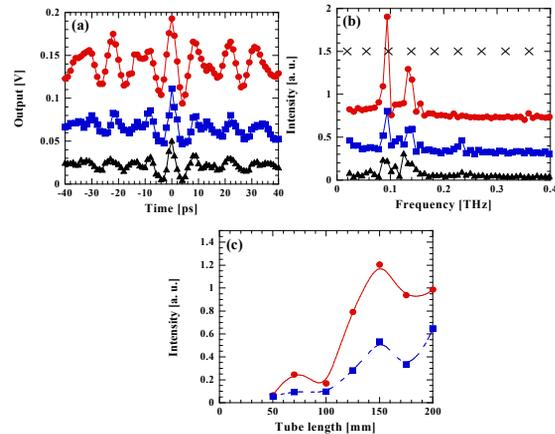
Figure 2: (a) Interferograms for 150, 100 and 50 mm tube lengths with offsets and factors adjusted for comparison. (b) Frequency spectra for 150, 100 and 50 mm tube lengths with offsets and factors adjusted. The theoretical
