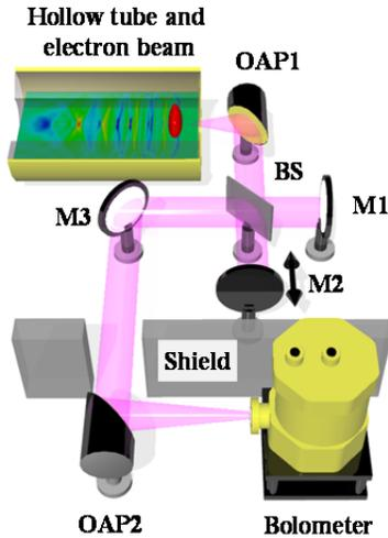
Figure 1: Diagram of multimode CCR and measurement system. OAP denotes an off-axis parabolic mirror; M, a plane mirror; BS, a beam splitter.
