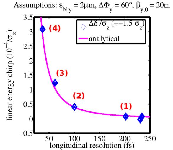
Figure 5: Measured linear energy chirp (diamonds) induced by the TDS as function of the longitudinal resolution together with the result of the analytical expression (magenta line) in Eq. (6).
