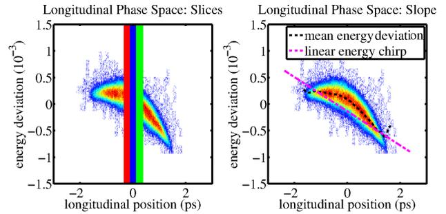
Figure 2: Data evaluation procedure for verification of the TDS-induced energy spread and linear chirp. Left: Three slices (colored) around the centroid with slice widths equal to the resolution. Right: Linear energy chirp between the mean energy at longitudinal positions of  $\pm 1.5\sigma_z$ .
