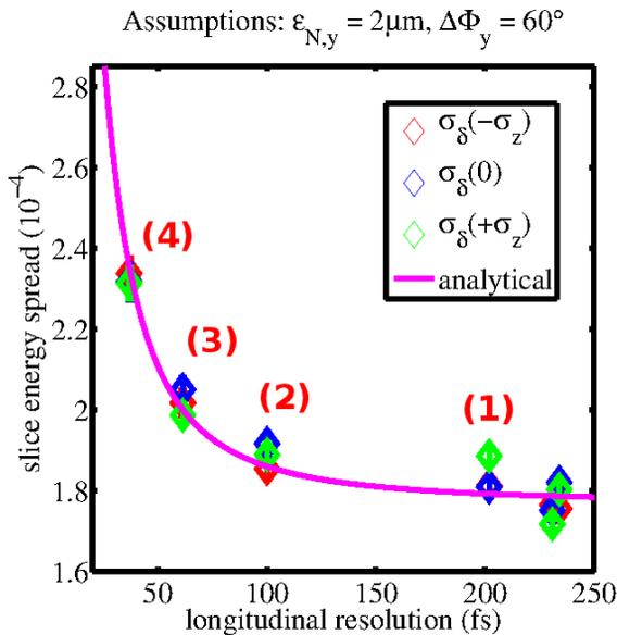
Figure 4: Measured slice energy spread (colored diamonds) for the three different slices around the centroid as function of longitudinal resolution together with the result of the analytical expression (magenta line) in Eq. (5).
