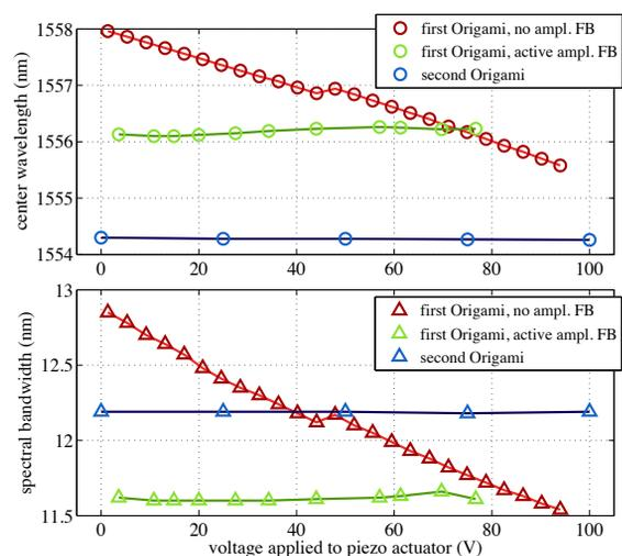
Figure 1: Comparison of the center wavelength (top) and the spectral bandwidth (bottom) of the two commercial laser systems as function of the voltage applied to the piezo actuator.
