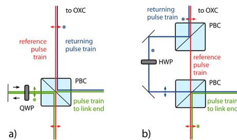
Figure 4: Optical path in the fiber link stabilization unit for splitting and recombining the pulse train into the reference and the one send to the link in a) the original and b) the upgraded units.
