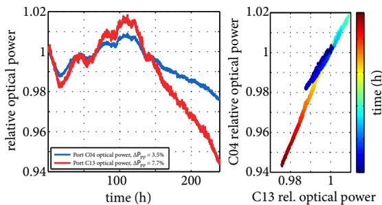
Figure 2: Drift of the optical power in the FSD over 10 days (left) and correlation of the two ports (right).
