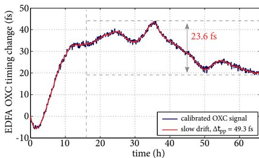
Figure 3: Timing drift of an EDFA connecting a fiber link unit to the free-space distribution unit.
