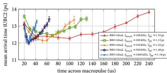
Figure 6: Bunch arrival time as function of the number of bunches in the macropulse at different repetition rates.
