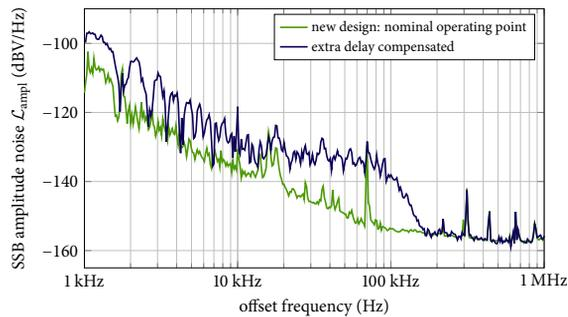
Figure 5: Single side-band amplitude noise measured at the “forward” optical power monitor in a link stabilization unit.
