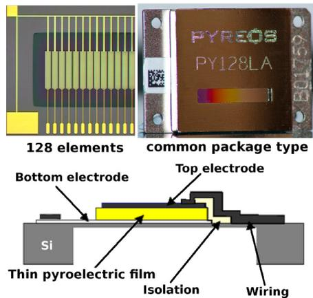
Figure 5: Line-array detector made of 128 thin pyroelectric film sensors [9]. Top: View on the single elements, and the entire detector unit with cut-out for the sensor array. Bottom: Sketch of the sensor assembly (cross section).
