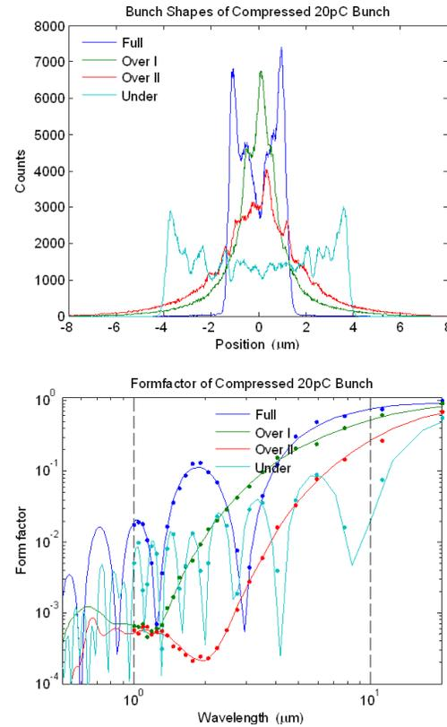
Figure 1: Simulations for ultra-short bunch operation with 20 pC bunch charge at LCLS. Top: Longitudinal bunch profile for different compression scenarios. Bottom: Corresponding longitudinal form factors, i.e. the information on the longitudinal profile in the frequency-domain.
