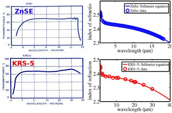
Figure 2: Transmission characteristics [5] and index of refraction according to data from literature [6, 7] and Sellmeier equation: ZnSe (top) and KRS-5 (bottom).
