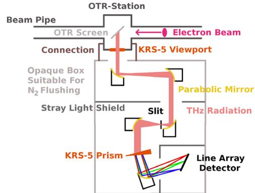
Figure 6: Prototype spectrometer layout for LCLS, including radiation transport optics and KRS-5 viewport.
