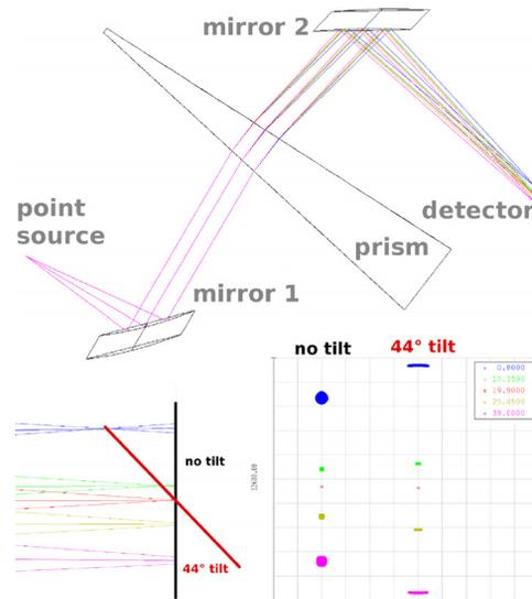
Figure 4: ZEMAX[8] simulation of the spectrometer configuration with KRS-5. The lower plots show the focal plane on the detector for different wavelengths (unit:  $\mu\text{m}$ ) and a detector tilted by  $44^\circ$  w.r.t the optical axis.
