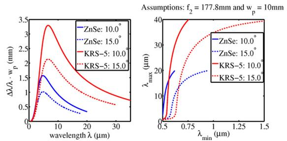
Figure 3: Spectrometer characteristics for different apex angles  $A$  of the ZnSe and KRS-5 prisms. Left: Wavelength resolution normalized to wavelength and radiation waist  $w_p$  at the prism. Right: Obtainable wavelength coverage from  $\lambda_{min}$  to  $\lambda_{max}$  with assumptions on  $f_2$  and  $w_p$ .
