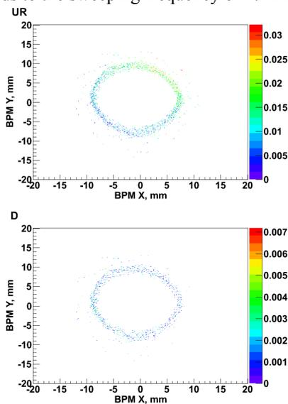
Figure 3: The signals (in V/nC) from a diamond (top) and a sapphire (bottom) sensor as a function of the beam positioning the azimuthal plane (as measured by the BPM). The bunch charge is 500 pC.
