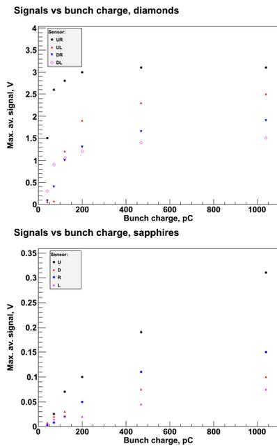
Figure 6: Signal from all diamonds (top) and all sapphires (bottom) as a function of the bunch charge in the machine.
