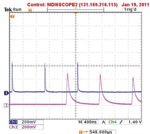
Figure 4: Signals from 3 bunches at FLASH: BLM #1 (top, HV=500V) and BLM #3 (HV=700V).
