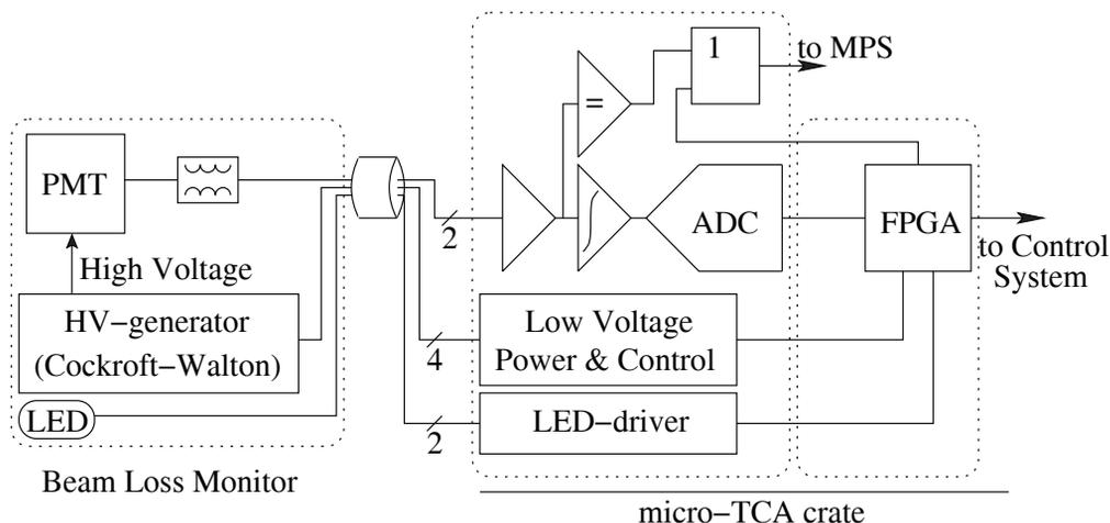
Figure 2: BLM signal processing chain.
