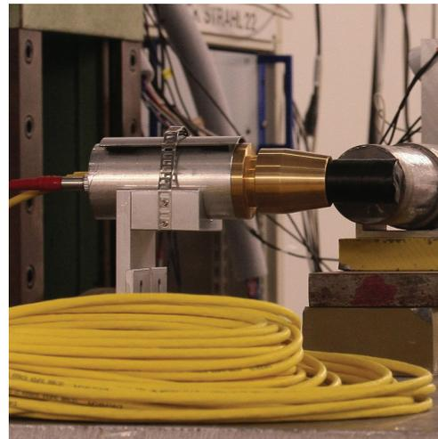
Figure 1: XFEL BLM prototype at DESY test-beam.
