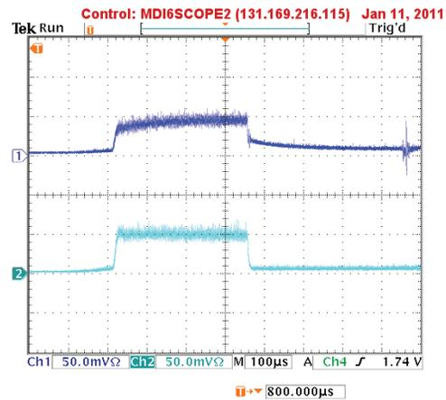
Figure 3: Signals from FLASH dark current: BLM #1 (top, HV=650V) and BLM #2 (HV=550V).
