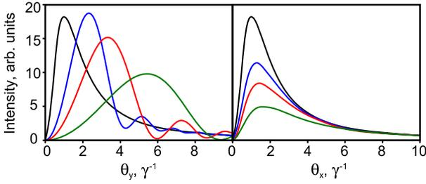
Figure 2: The angular distributions of the BTR from different targets: black curve – flat target, blue curve – cylindrical target  $R = 50$  mm, red curve – cylindrical target  $R = 25$  mm, green curve – cylindrical target  $R = 10$  mm.
