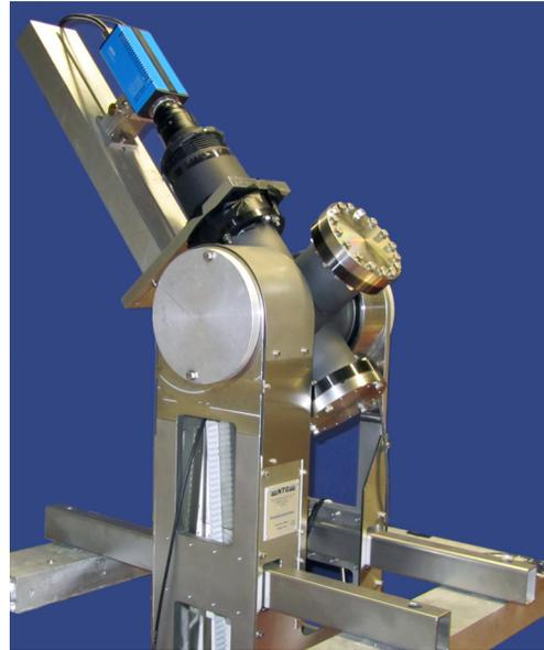
Figure 1: Test stand for optical beam tomography.
