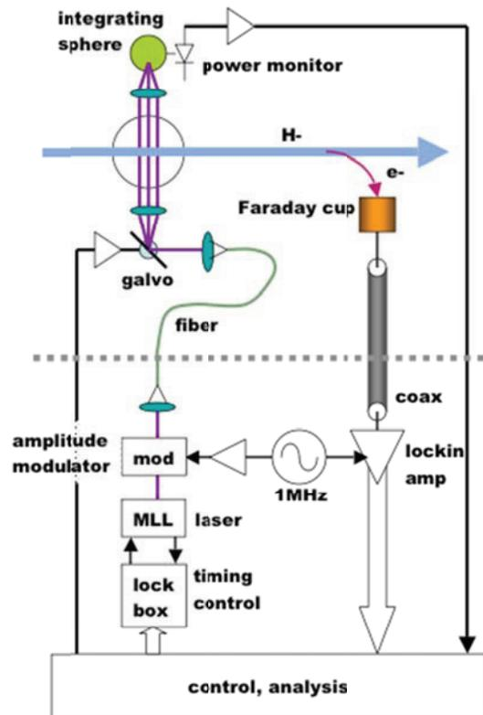
Figure 1: Laser wire block diagram.
