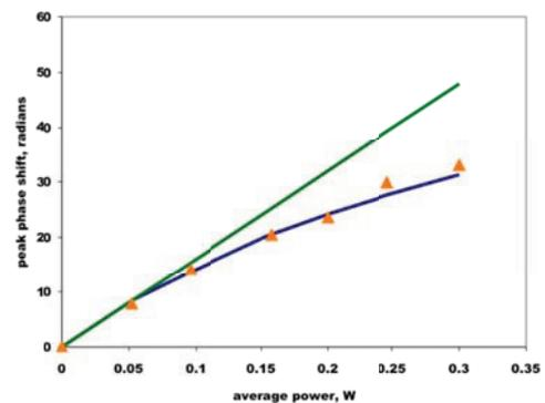
Figure 3: Peak phase shift versus transmitted power from experiment and from model.
