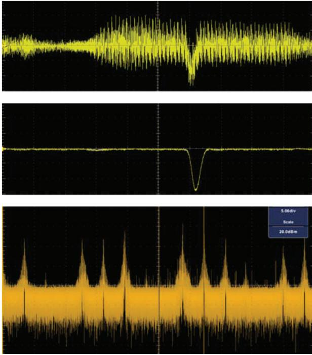
Figure 2: Noise on SNS laser wire in time domain (a), low pass filtered (b) and FFT of a 10us section of noise (c). Upper traces: 20mV/div., 100ns/div. Lower trace: 20dB/div., 125MHz/div.
