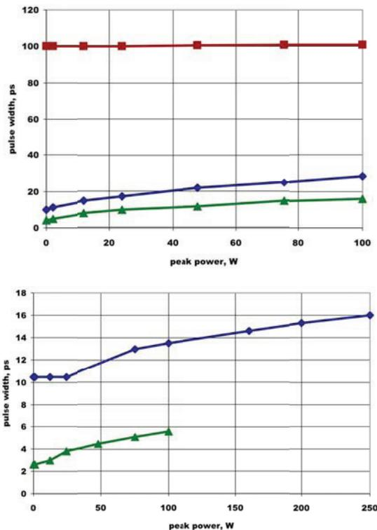
Figure 4: Model results for different pulse lengths and 100m fiber (a), 30m fiber (b), versus power.
