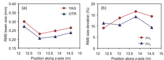
Figure 4: (a) Geometric RMS beam size measured with YAG and OTR screens at different locations. (b) Horizontal and vertical RMS size deviation ( $\Delta\sigma_x$ ,  $\Delta\sigma_y$ ) between the measurements with YAG and OTR screen. The beam momentum was 24.8 MeV/c and quadrupole fields were applied.
