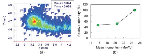
Figure 3: (a) Beam image measured with Ce:YAG coated powder screen at 1.76 m downstream a vertical 10  $\mu\text{m}$  slit position for electron momentum of 14.7 MeV/c. (b) Measured relative intensity of the OTR light as a function of beam momentum.
