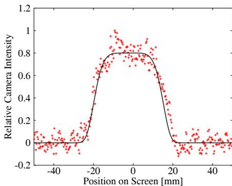
Figure 8: Transverse profile measured with a 5 ns gate.
