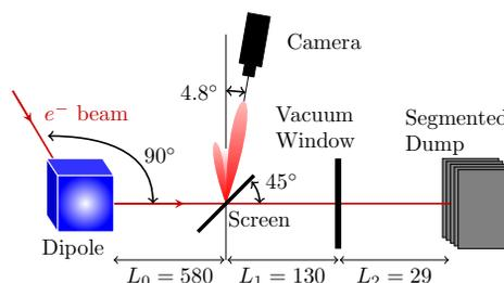
Figure 1: Layout (in mm) of the PHIN spectrometer.
