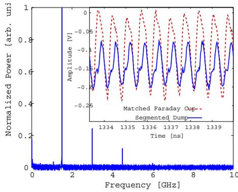
Figure 6: Individual bunches measured by the segmented dump and the FFT of the pulse.
