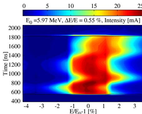
Figure 2: Time resolved energy spread; the energy fluctuations along the pulse are due to RF variations [6].
