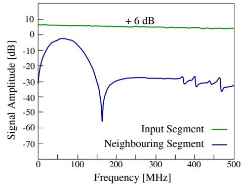
Figure 3: Crosstalk measured with a network analyser.
