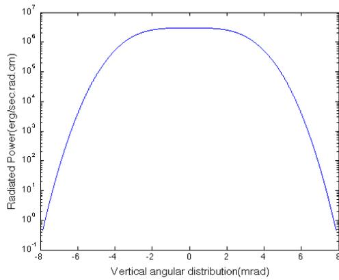
Figure 2: Angular distribution of the SR from the bending magnet (Energy=1.3GeV, Bending radius = 3.9m, Wave length ( $\lambda$ )=500nm, Sigma-mode polarization).
