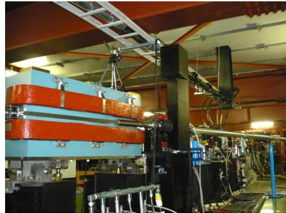
Figure 4: Picture of the SR line; The visible light of the SR is guided by using three mirrors in the accelerator room. The mirrors are set in the black duct to avoid the background light.
