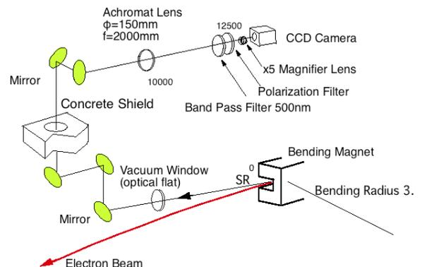
Figure 1: Layout of the EXT-SR monitor.
