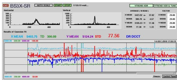
Figure 6: time trend of the beam profile in 10 minutes. Plots show the vertical beam size, the horizontal beam size, the vertical beam position, the horizontal beam position and DR current measured by DCCT.
