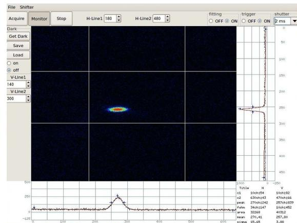
Figure 5: example of the acquired beam profile; the beam size is calculated from the fitting of the projected image in horizontal and in vertical. Two lines at both side of the image are integration area to calculate the projection.
