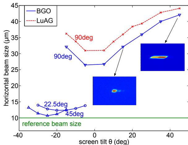
Figure 4: Horizontal beam size of simulated images from BGO (blue) and LuAG (red) screens. The angles between camera and incoming beam are  $22.5^\circ$ ,  $45^\circ$  and  $90^\circ$ , respectively. Two images from test experiments are included.
