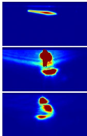
Figure 1: Top: Beam image without COTR (LuAG screen). Middle and bottom: Strong COTR effects lead to saturation in the beam images (OTR screen with shortpass and long-pass filters). For more details see Ref. [5].
