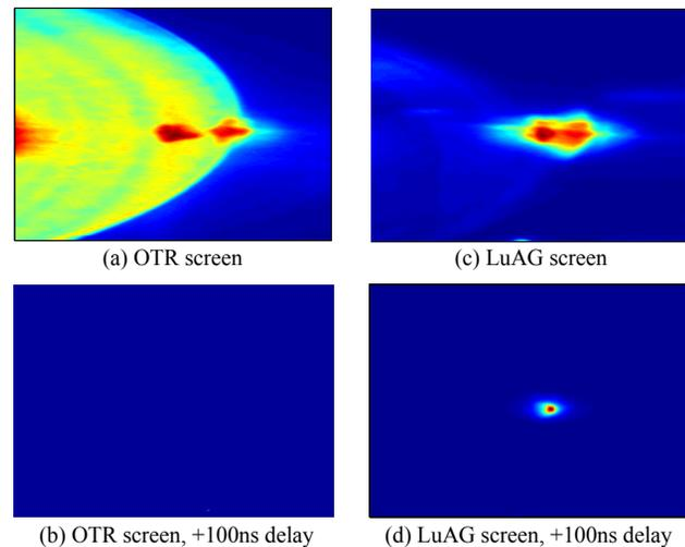
Figure 3: Camera images of the beam with (a) OTR screen, (b) OTR screen with 100 ns camera delay, (c) LuAG screen, (d) LuAG screen with 100 ns camera delay.
