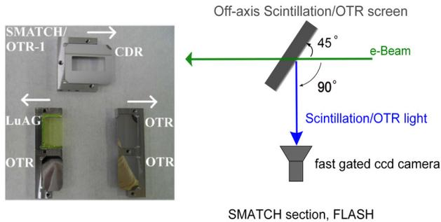
Figure 2: Left: Screen holder with imaging screens at diagnostics section SMATCH; emission directions indicated by arrows [5]. Right: Top view of the layout of the experimental setup.
