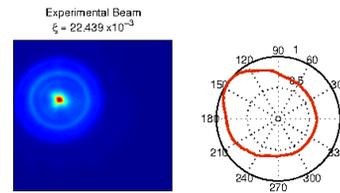
Figure 4: The measured beam as cumulated slice with its symmetry characteristics. Note, that the middle of the polarplot is the center of gravity, not the middle of the image.
