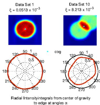
Figure 3: Comparison of the symmetry characteristics of the cumulated slice of data set 1 and data set 10.
