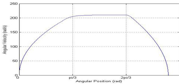
Figure 4: Angular speed vs angular position of the motor.
