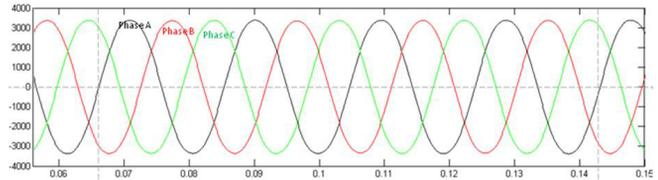
Figure 7: Measured Electromotive force (EMF) voltage of 3 phases.
