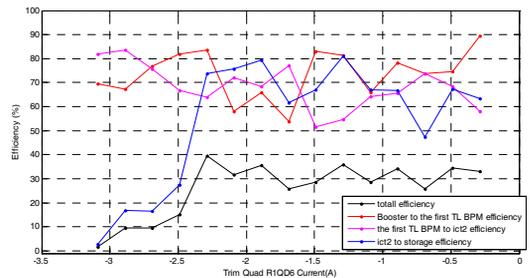
Figure 10: Trim quadrupole R1QDT16 effects on efficiency.
