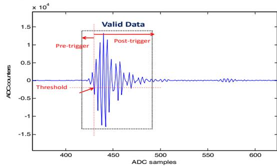
Figure 1: Three parameters defined to calculate position.
