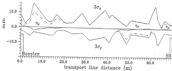
Figure 7: Optical function of Booster to the Storage Ring Transport Line.
