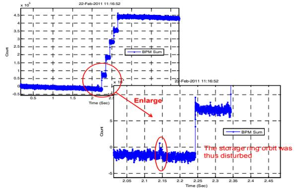
Figure 5: R1BPM3 10 kHz sum readout. The red circle of the below picture remarks that booster has no current but pulse magnet still fired caused the orbit disturbed.
