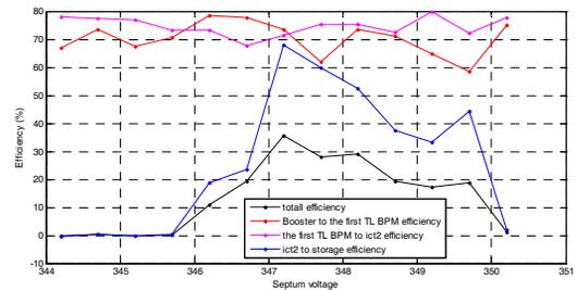
Figure 9: Septum charging voltage effects on efficiency.
