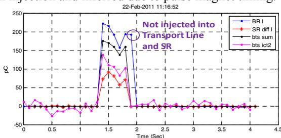
Figure 4: Booster, Transport line BPM sum and DCCT and Storage ring charges during top-up injection.
