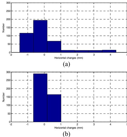
Figure 8: (a) LTB BPM1 (high dispersion) horizontal position change. (b) LTB BPM4 (low dispersion) horizontal position change.
