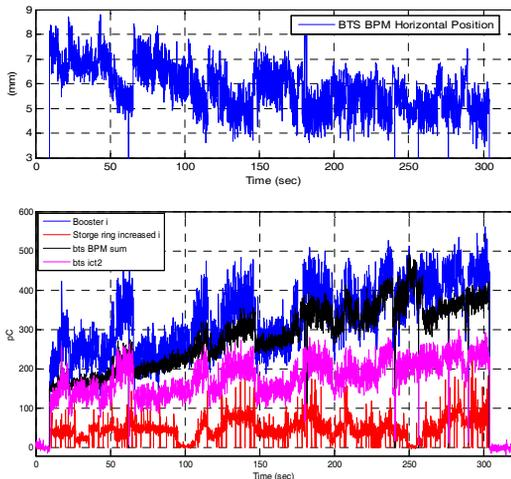
Figure 3: Booster, BTS BPM sum and hor. position and DCCT and Storage ring increased charges.
