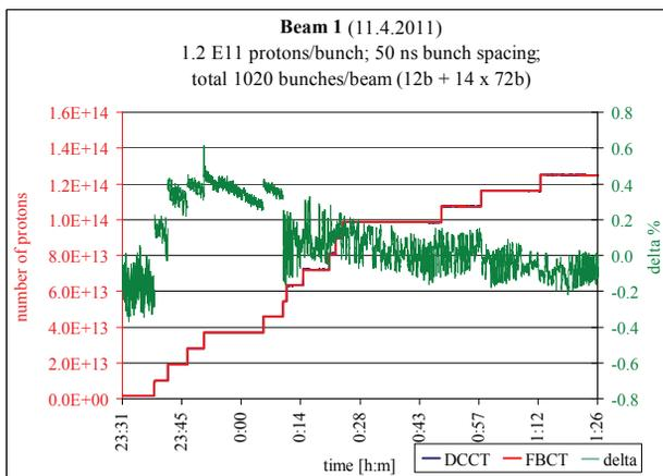
Figure 6: BCTs reading during a scrubbing run (highest number of bunches injected so far)
