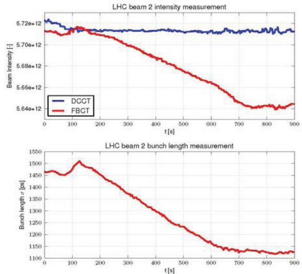
Figure 4: FBCT readings decrease with bunch length during the ramp while DCCT behaves correctly.
