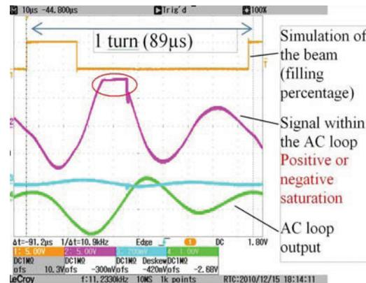
Figure 2: Plot showing a positive saturation of the 2010 AC loop with a given filling pattern simulated on the test bench.
