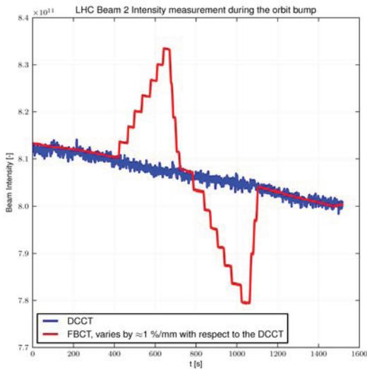
Figure 3: FBCT readings vary during controlled orbit bumps at the location of the FBCTs and DCCTs.
