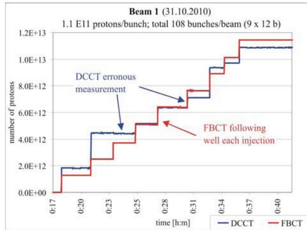
Figure 1: DCCT dependency on the filling pattern.
