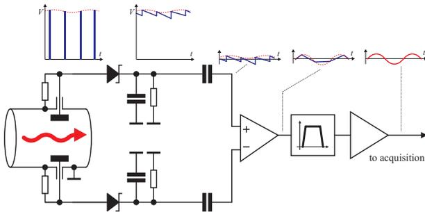
Figure 1: Schematic BBQ block diagram.
