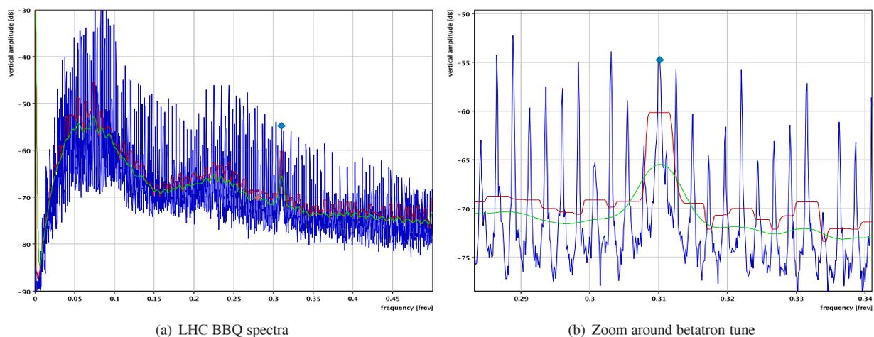
Figure 3: Raw ( $|S_{raw}(f)|$ , blue), intermediate median- ( $|S_{med}(f)|$ , red) and low-pass filtered magnitude spectra ( $|S_{lp}(f)|$ , green) as used in the revised tune fitter algorithm.
