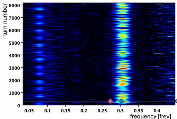
Figure 4: BBQ Wavelet spectrum. The burst-type character of the tune oscillations at  $Q_y = 0.31$  is visible.
