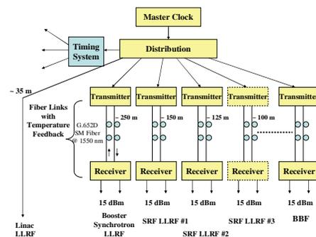
Figure 3: RF reference distribution scheme for the TPS.
