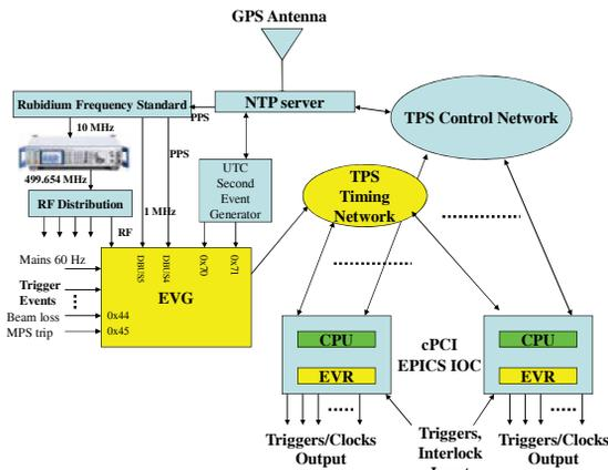
Figure 4: Block diagram of the TPS event system.
