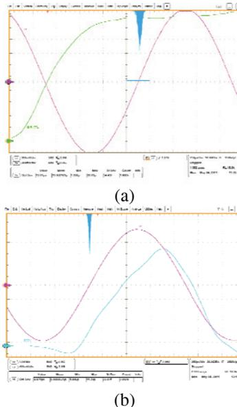
Figure 8: (a) Jitter of the cPCI-EVR-300 TTL output relative to the RF clock and (b) Jitter of the beam relative to the RF clock. The beam is triggered by combination of the cPCI-EVRTG-300 and GUN-RC-203 trigger module.
