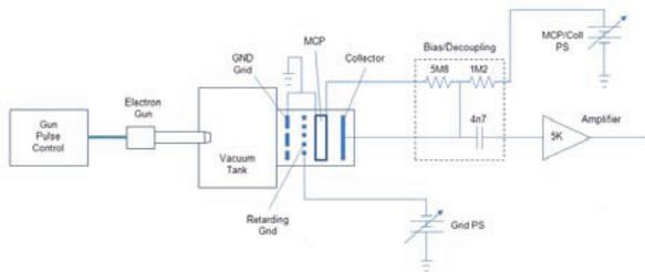
Figure 2: A schematic diagram of the detector characterization setup.
