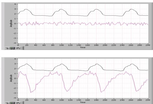
Figures 6 and 7: MCP version detector signals. The screenshot on the top was taken with 200V applied to the retarding grid and the one on the bottom without any potential applied. The black trace is the beam position monitor sum signal and the purple one is the electron cloud signal with a vertical scale of 10mV/div.
