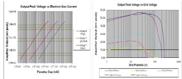
Figures 3 and 4: Left: Full system (detector and amplifier) transfer functions corresponding to three different MCP gains. Right: Graph showing the amplifier output signal versus retarding grid potential for five different electron energies at a constant beam current.
