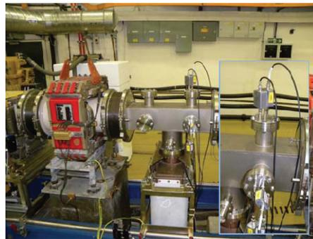
Figure 5: Detail of the installed detectors at the ISIS straight 5 location.
