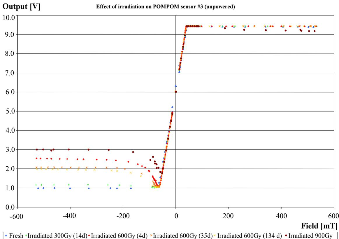
Figure 3: Effect of successive 300 Gy irradiations (<sup>60</sup>Co) on sensor #3. Intervals between exposure and measurement are given in days, where relevant. The immediate effects of the second dose (to 600 Gy) abate within a few weeks, but the remaining damage lasts for months. The final (900 Gy) results were taken just a few hours after the irradiation; the scatter is from the real changes in device response with time as it recovers.
