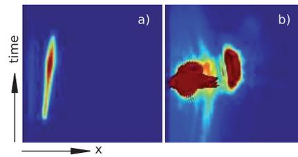
Figure 6: Images of a TDS streaked electron bunch at FLASH. While a) seems to be free from COTR effects, b) is COTR dominated. Between a) and b) the phase of the accelerating module ACC1 in front of the first compressor chicane was changed by  $0.5 \text{ deg}$ .
