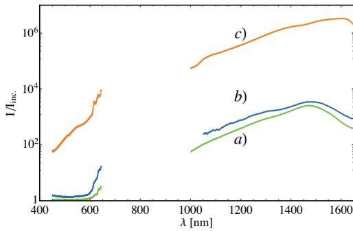
Figure 8: CTR spectra in the VIS and NIR regime observed at FLASH for three different compression modes: a) on-crest, b) moderate compression, c) partially overcompressed. The longitudinal phase space distribution of these settings is shown in Fig. 9.
