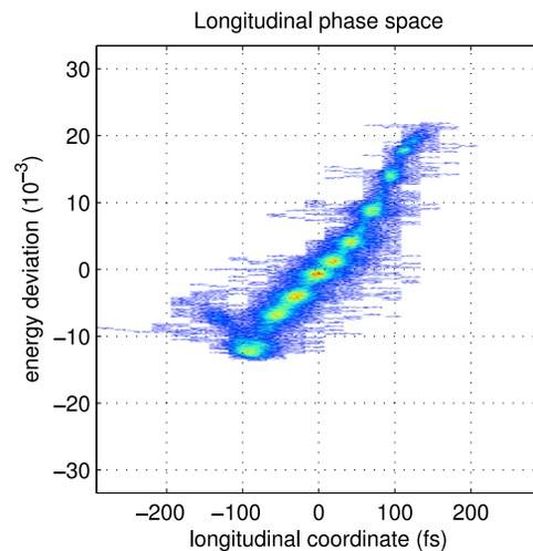
Figure 7: Longitudinal phase space of a compressed electron bunch at FLASH imaged using the transverse deflecting structure (TDS) and a dispersive dipole. The bunch exhibits substructure in energy and longitudinal coordinate at a scale of  $20 \text{ fs}$  but produces no COTR effects.
