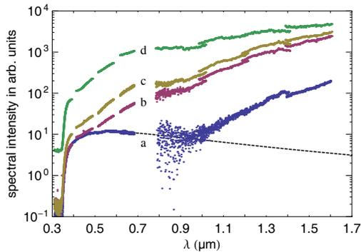
Figure 5: CTR spectra in the VIS and NIR regime observed at FLASH in front of the energy collimator. a) normal FEL operation (non-linear compression), b) - d) on-crest operation of ACC1 with different strengths of the compressor chicanes [9].
