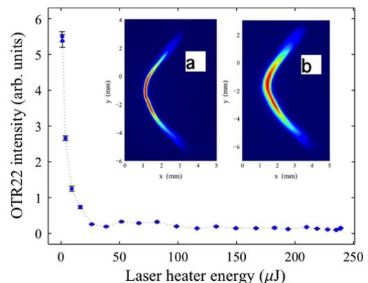
Figure 10: COTR intensity as function of laser heater power at LCLS. The phase space for no heating (a) and normal operation heating (b) are shown in the inset.
