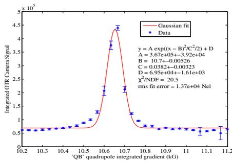
Figure 2: Integrated CTR intensity observed at LCLS after DL1 as function of QB quadrupole strength [5].
