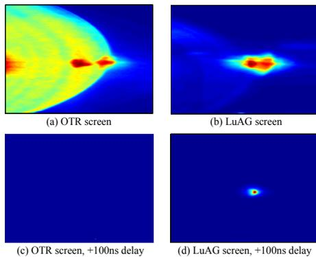
Figure 11: Imaging electron bunches at FLASH using a scintillator screen and fast gated intensified camera [23]. The prompt OTR image (a) exhibits severe COTR/COSR effects as does the prompt image from the scintillator (LuAG) screen (b) which is dominated by surface COTR. With a gate delay of 100 ns, the OTR image vanishes completely while the scintillator afterglow reveals the true bunch shape.
